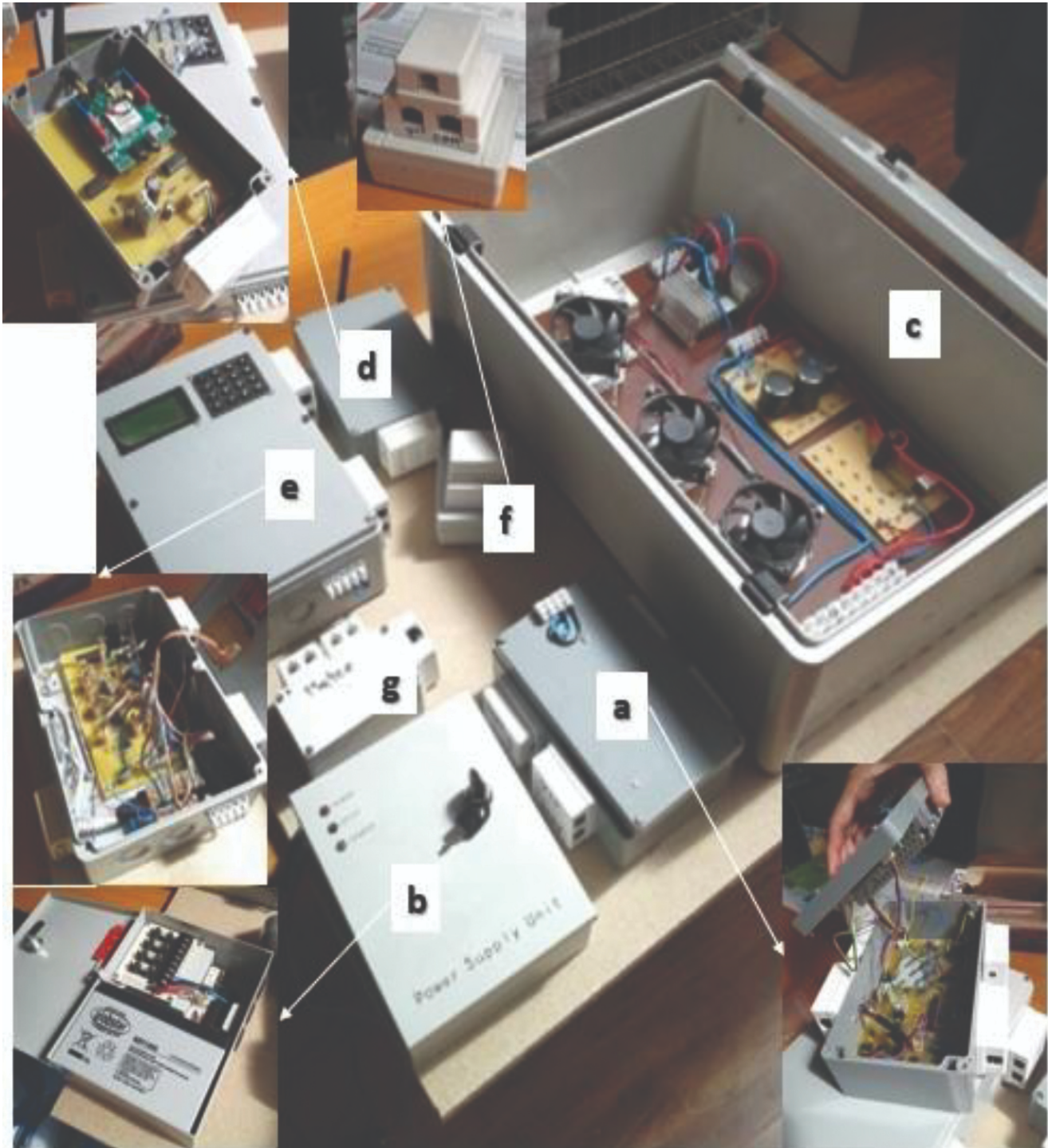
Figure 11: Lenz wind-turbine electronics.
