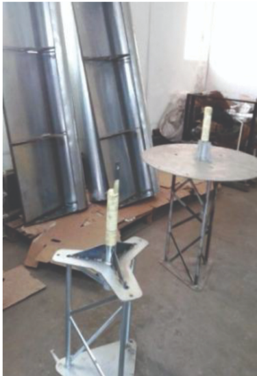
Figure 9: Blades and upper parts from the main pillar before and after the painting procedure.
