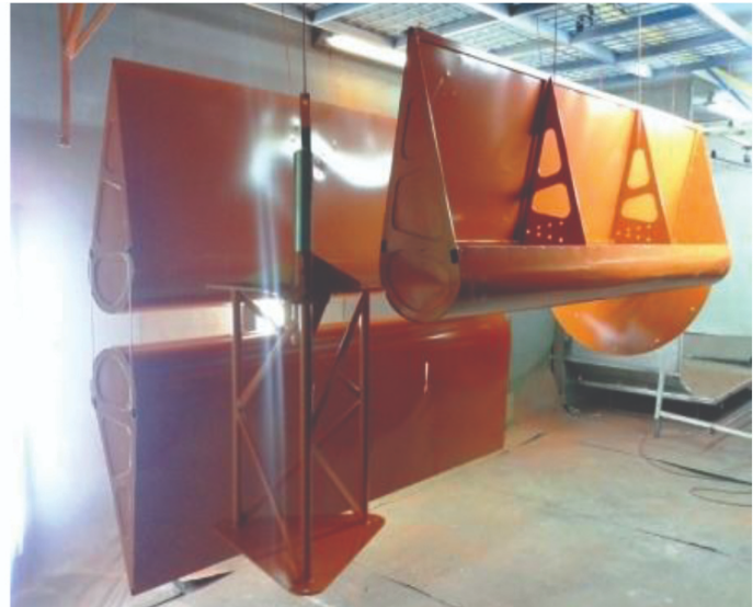
Figure 9: Blades and upper parts from the main pillar before and after the painting procedure.
