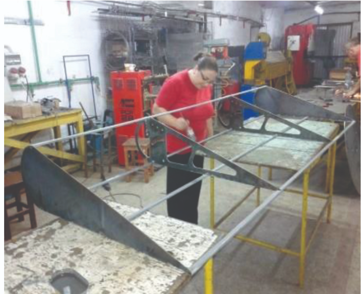
Figure 8: Turbine towers (left) and blade (right) after applying the protective zinc coat.
