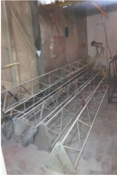
Figure 8: Turbine towers (left) and blade (right) after applying the protective zinc coat.
