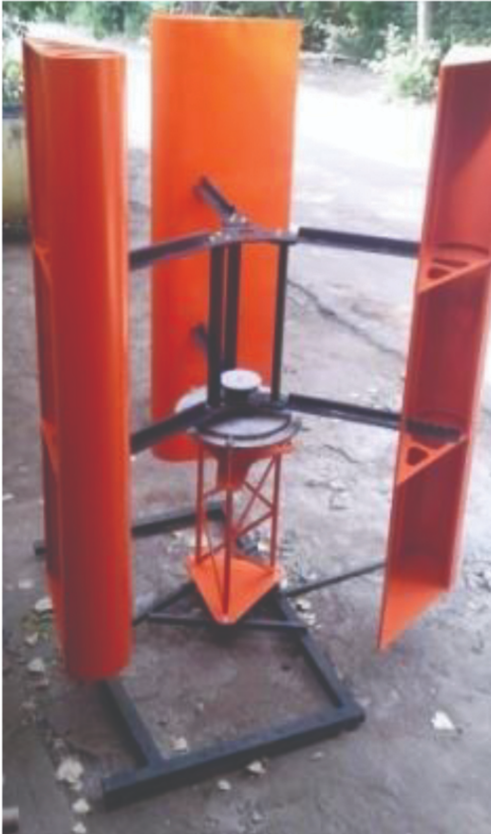
Figure 12: Lenz turbine assembly.
