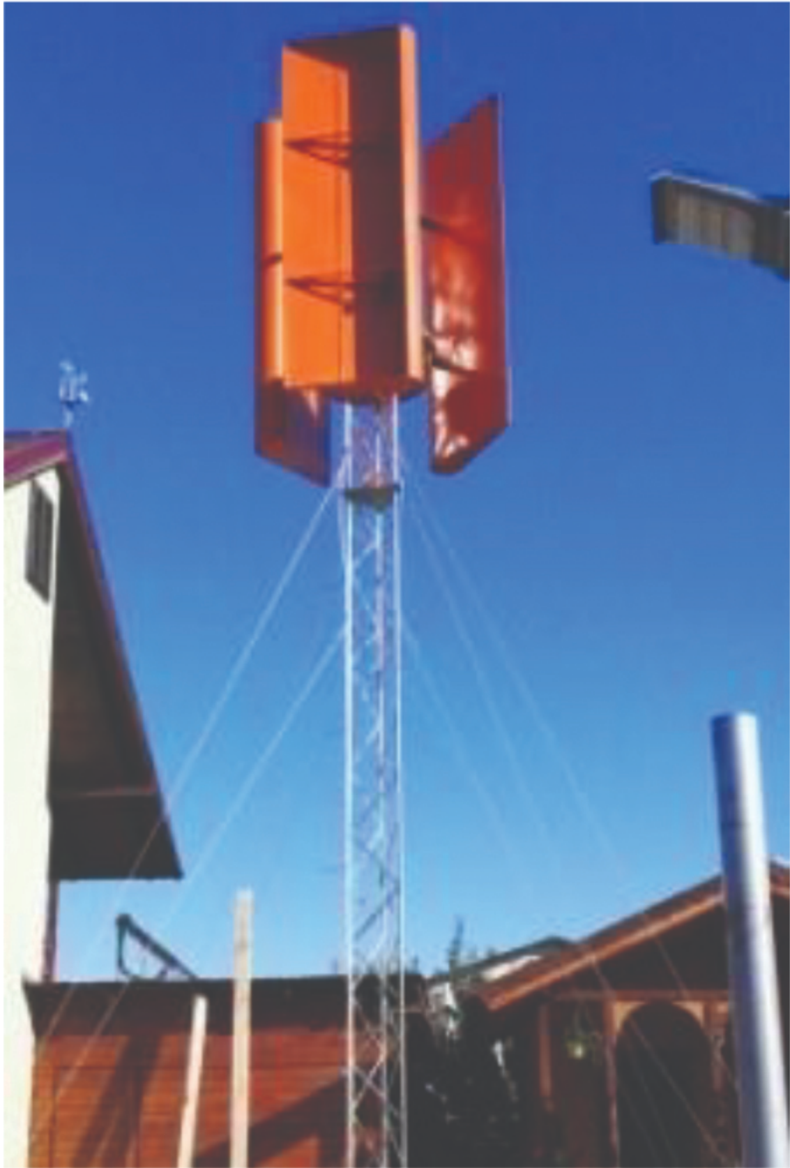
Figure 14: Lenz wind-turbine installed.
